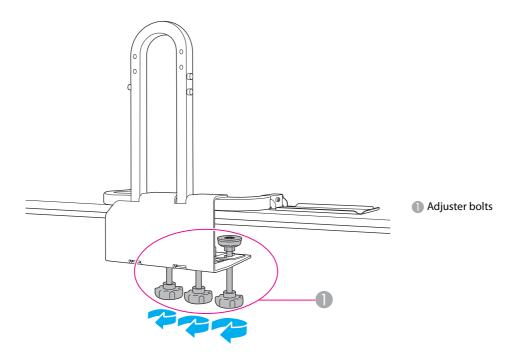
(2) Attach the base frame unit to the table by sliding the base frame unit onto the edge of the table.
