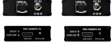
The PRO-HDMIFO-KIT is a Transmitter and Receiver set for sending HDMI signals over long distances via Fiber Optic cabling. Connect a HDMI source to the Transmitter unit and the uncompressed signal will be passed over fiber optic to the Receiver where it is outputted as HDMI for connection to the display. HDMI Transmission distances of up to 300m can be achieved using this advanced fiber optic technology.
