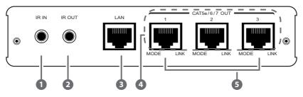
**1** IR IN: Connect with IR Extender to receive IR signal from Transmitter side and blast out at Receiver side. Ensure that remote controller being used is within he direct line-of-sight of the IR Extender.
