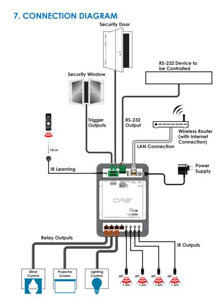
**Note:** The IR input is also used for IR learning. When using the IR learning function, please hold the remote control's IR emitter no more than 15cm from the IR input's receiver to ensure that the signal can be captured properly.
