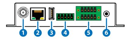
**1 DC 5V:** Plug the 5V DC power adapter into the unit and connect it to an AC wall outlet for power.
