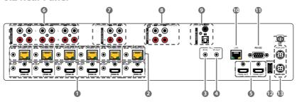
1 HDMI IN & IR OUT 1~6: Connect up to 6 source devices to the HDMI ports using appropriate quality HDMI cables. Input source devices include Blu-ray players, set-top boxes, game systems and so on. These inputs are DVI-D compliant (with the use of DVI to HDMI adapters or cables). Attach IR blasters to the IR Out ports to transmit the IR signals received from connected HDBaseT Receivers. The IR signal routing follows the HDMI signal routing.
