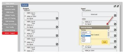
**Timing:** Test patterns can be generated with the following standard timings: 720p@50/60Hz, 1080p@50/60Hz, 4K@25/30Hz. Test pattern output does not use HDCP.
