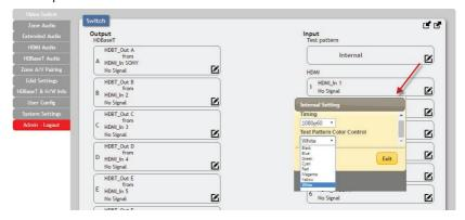
**Colour**: The test pattern can be changed to any one of a choice of eight colours.
