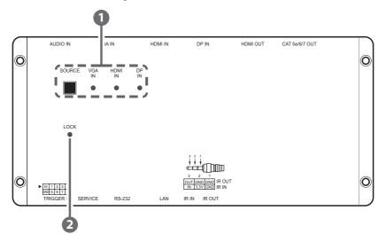
1 SOURCE & LEDs: Press this button to sequentially switch through the available inputs. The LED will illuminate GREEN to indicate which source is currently selected. Live, but unselected, sources will be lit RED.
