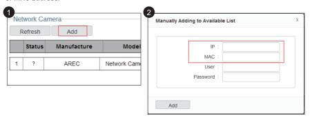
Step 5 : Connect to devices Status of refreshed or added device displays symbol "?". Click web cam and auto tracking cloud and the device setup page displays. Enter Administrator and Password to change devicestatus, press OK to save your changes and exit.
