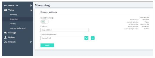
Live streaming: Select ON/OFF to enable/ disable live streaming ability. Protocol — The available protocol on the LS-300 are RTP and RTMP.
