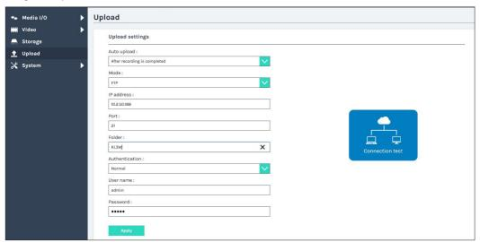
Auto upload- Select from the drop-down list. Start uploading "after recording is completed", or turn "OFF" the function. Followings to be configured according to the upload destination.
