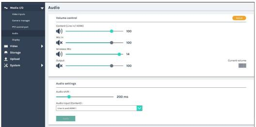
Volume control- Tune the recorded volume from each audio input and adjust the audio output volume. Configurable range of sound input is 0-125, of AREC wireless microphone 0~15. The nearby volume meter indicates the encoded audio volume. Audio settings- Set AV synchronization and configure the source from each audio input.
