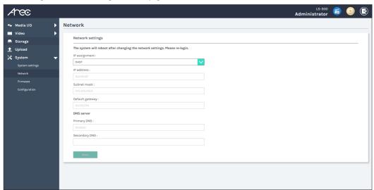
IP assignment – Select DHCP to have IP address be allocated by a router or any DHCP server being connected; or Select Static IP and enter the required network settings including IP address / subnet mask / default gateway/ DNS server.
