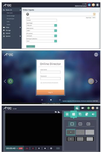
The Online director allows user to control recording and have a live stream view of the output video. The control panel makes it easy to apply layout, select background, and control the audio recorded during the recording process.
