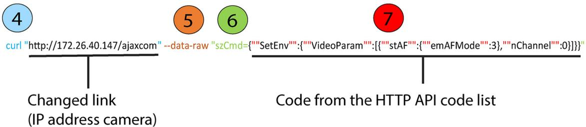
8. Modify the parameters in the code. In the example above **EmAFmode:3** and **nChannel:0** See the [HTTP API code list](#).
