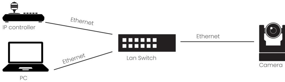
Figure 13: IP Network Connection Diagram
