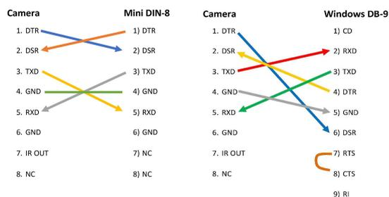
Figure 8: RS-232 Interface (Mini DIN-8)
