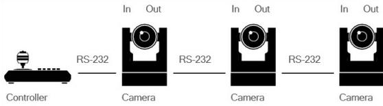
Figure 10: RS-232 Network Connection Diagram
