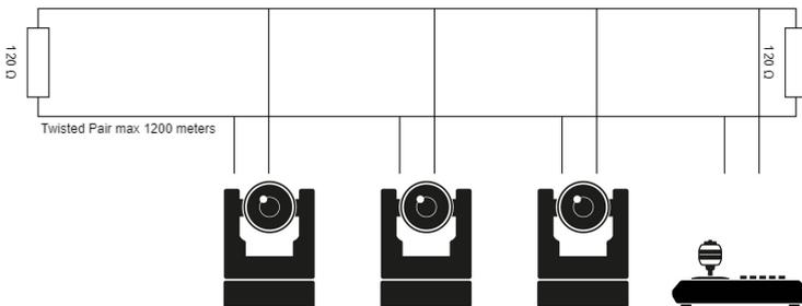
Figure 12: RS-485 Network Connection Diagram
