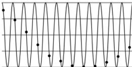
In this example, the dots represent the sampled data and the curve represents the original signal. Because there are not enough sampled data points, the resulting pattern produced by the sampled data is a poor representation of the original.
