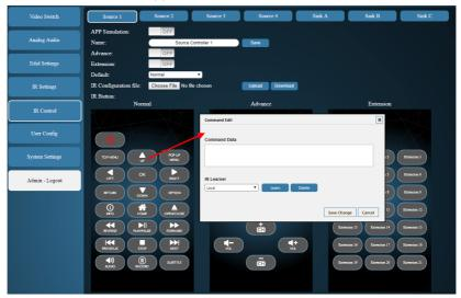
■ **Key Name ("Extension" and "Source Controller" buttons only):** Allows renaming the current button for easy identification. Type the new name in the space provided. The name can be up to 32 characters long.
