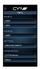
■ **HDMI:** Select this to control the display connected to Output C (HDMI) and the currently routed input. After selection, the app will automatically return to the Main page.
