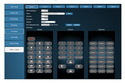
1) **Source 1~4/Sink A~C Buttons:** Press the button of the Source or Sink that you wish to configure the IR commands for.
