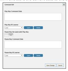
■ Play Key Command Data: Contains the IR command data to be transmitted when the PLAY/PAUSE button is pressed. This data can be learned from an external remote or manually entered.
