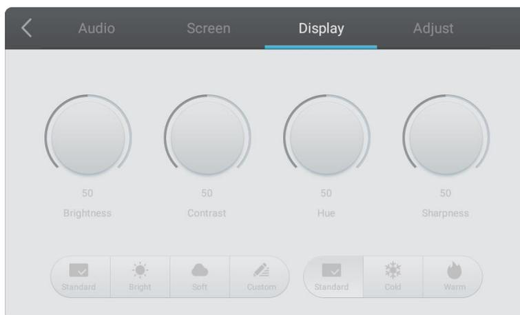
Select a preset configuration to adjust the brightness, contrast, hue, and sharpness of the image, or manually set a custom configuration.
