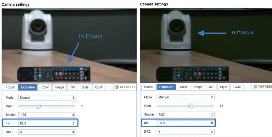
Figure 25: Exposure > Manual with Iris F2.0 (left) and Iris F6.8 (right)
