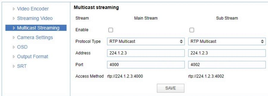
Figure 19: WebGUI > VIDEO > Multicast Streaming
