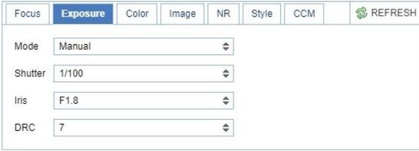
Figure 24: WebGUI > VIDEO > Camera Settings > Manual Exposure Mode
