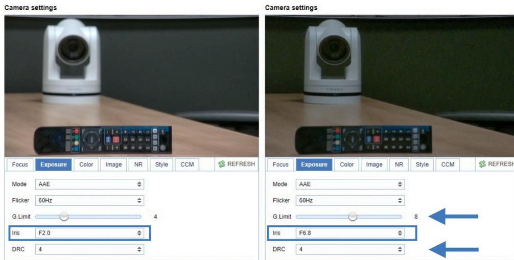
Figure 27: Exposure > AAE with Iris F1.8 (left) and Iris F6.8 (right)
