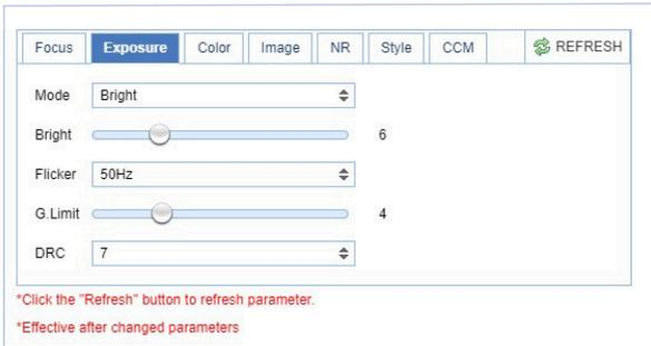
Figure 28: WebGUI > VIDEO > Camera Settings > Bright Exposure Mode
