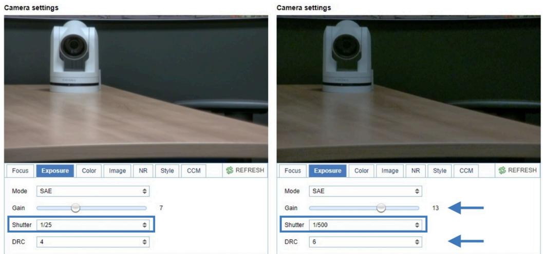
Figure 26: Exposure > Shutter speed at 1/25 (left) and 1/500 (right)
