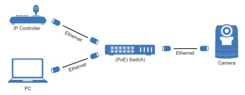
Figure 13: IP Network Connection Diagram
