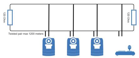
Figure 12: RS-485 Network Connection Diagram
