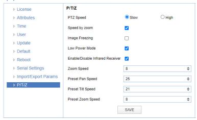
Figure 49: WebGUI > SYSTEM > P/T/Z
