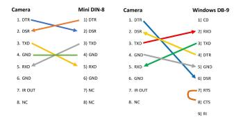
Figure 8: RS-232 Interface (Mini DIN-8)
