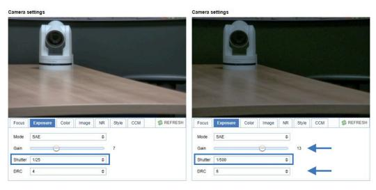
Figure 26: Exposure > Shutter speed at 1/25 (left) and 1/500 (right)
