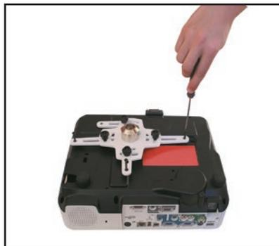
4. Secure the adjustable arm plate to the projector by positioning the plate's screws with the designated holes on the bottom of the projector.
