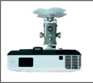
5. Secure the projector to the ceiling mount with the two setscrews.
