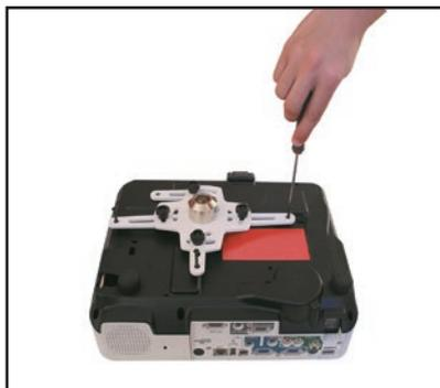
4. Secure the adjustable arm plate to the projector by positioning the plate's screws in the designated holes on the bottom of the projector.
