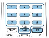
Remote control operations for the projector with the selected ID are enabled.
