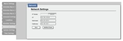
1) Network Settings: IP mode may be switched between Static IP or DHCP. In Static IP mode the IP, netmask and gateway addresses may be manually set. When in DHCP mode, the unit will attempt to connect to a local DHCP server and obtain IP, netmask and gateway addresses automatically. Please press "Save" after making any changes to the IP configuration or mode. To return all network settings to their defaults, press the "Network Reset" button.
